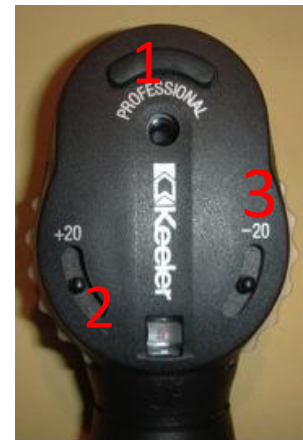
Fig 1: The Direct Ophthalmoscope. The operator side showing the viewing aperture (1), the lens indicator (2) and the rotating carousel housing the lenses (3)
