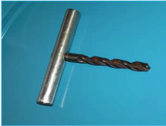
Figure 3. Modified drill bit for creation of an osteotomy
